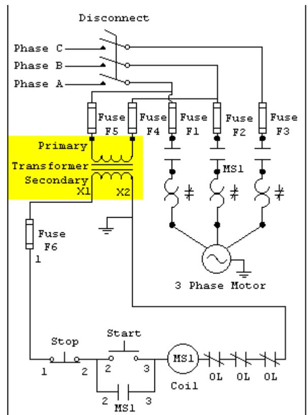
100VA transformer must be 8/10 Amp or smaller. A fast acting fuse is best. Refer to the NEC.
