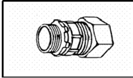
**Figure 4-2. Three-piece fitting**
