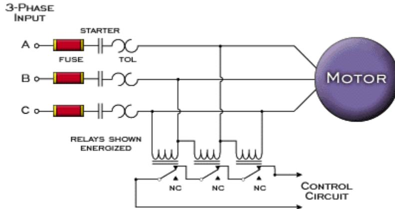
Three-phase motor single-phasing protection can be provided by time-delay overcurrent protection fuses sized at 125 percent of the motor running current. To produce rated torque under single-phasing conditions, motors will draw a line current of 173 to 200 percent of normal. The overload devices will open to protect the machine in this case. However, this will occur only where the motors are being operated at or near their nameplate ratings.
