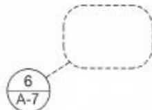
The detail symbol is used to indicate where a portion of construction is drawn to a larger scale. A circle or rectangle is placed around this part on a drawing.
