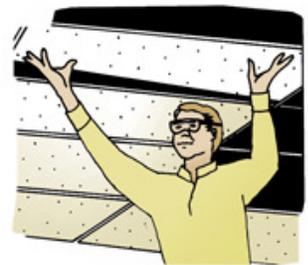
Figure 17 Tilt the ceiling panels slightly and drop them into position.
