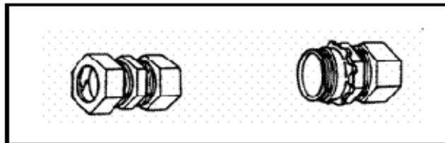
**Figure 4-7. Threadless couplings and connectors**
