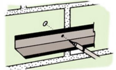
FIG. 7 - Fasten the wall angles securely to the wall at all points
