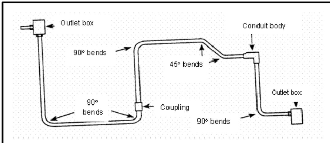
**Figure 4-13. Conduit body usage**
